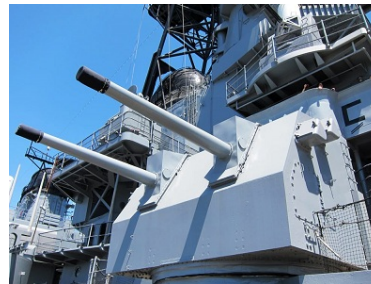
5 inch 38 cal Mark 12 Anti-Aircraft/Dual Purpose Gun
